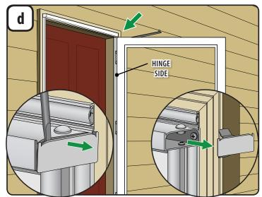
Identify the hinge side of your door. Using a flat blade screwdriver, separate the hinge side endcap from the rain cap assembly and firmly pull sideways until it is completely removed. Set aside endcap for later use.
