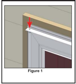
In this step, you will remove the old latch rail from the mounting surface.
